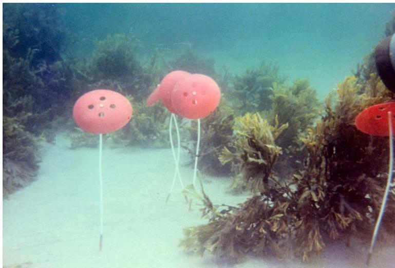
**Figure 6.** Cefas Mushroom Drifters floating along the seabed.
