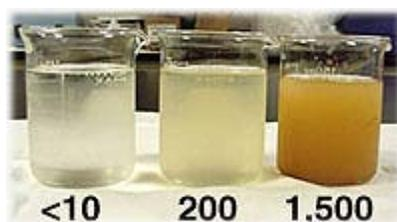
**Figure 9.** Turbidity of <10 NTU, 200 NTU and 1,500 NTU.
